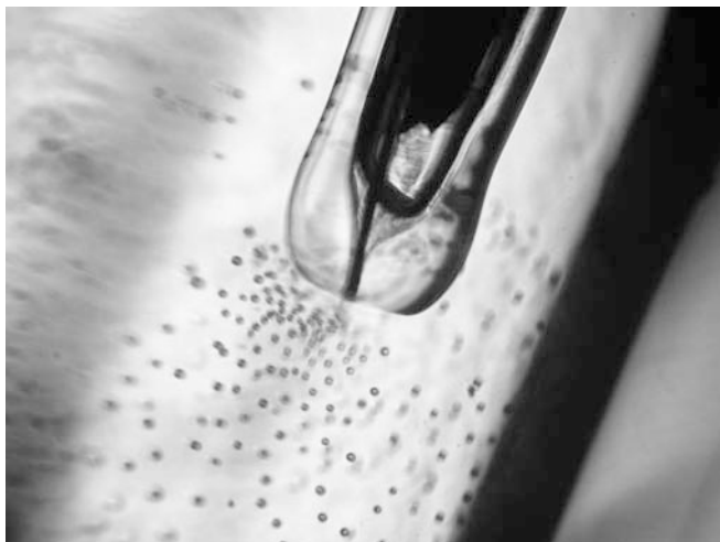
Fig. 7 Evolution of microbubbles of gas during electrooxidation of undiluted methanol at Pt microelectrode. The picture was taken as the voltammogram entered the region of current oscillations (circa 4.3 V vs Pt quasi reference electrode). Radius of Pt microdisk: 10 \mu\text{m} ; T=22\text{ }^\circ\text{C}
